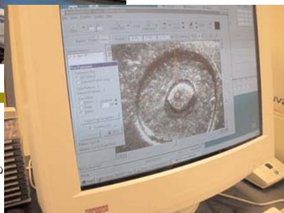
to 50 microns (0.025 to 0.050mm) in diameter and depth. The hole, although small, can be barely be seen by the naked eye, which has caused concern among collectors. Thus, this method has yet to be accepted for use on coins by a number of collectors. We feel that this will be the method of choice in the future for analyzing and certifying of ingots and coins. The quality of information will more than
